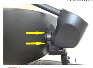
**STEP 3** - When the mount is positioned as far forrward as it will go, tighten the clamp screw untill the Top and Mid Sections are **slightly snug** around the mirror stem. You should still be able to rotate the mount.
